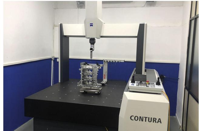
**Figure 2.** Coordinate measuring machine (CMM Contura G2 10/16/06 RDS; Carl Zeiss Industrielle Messtechnik GmbH) analysis.
